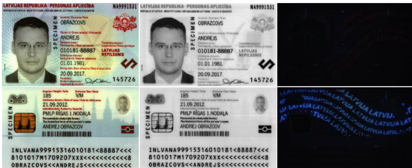
Duplex scanning of documents. The front and back of an identity card in white, infrared, ultraviolet lights
